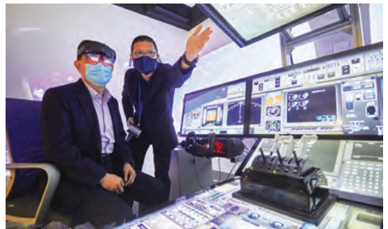
The Lab includes a cockpit with Augmented Reality and Virtual Reality (VR) technology to train pilots to respond to a range of simulated scenarios. Photo: National University of Singapore
