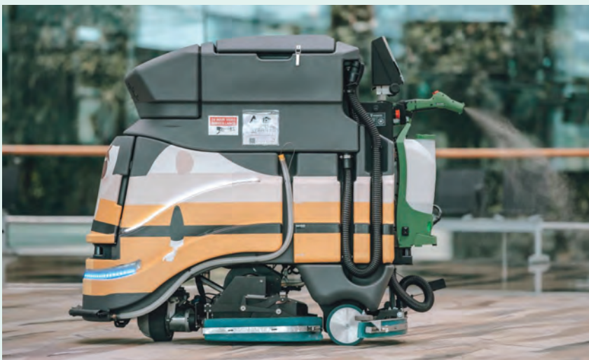
Autonomous cleaning robots used in Changi Airport's terminals have been equipped with a misting attachment that disinfects the carpets immediately after cleaning. Photo: Changi Airport Group
